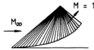
Figure 5.15 Isentropic compression (reversed Prandtl Meyer expansion).
