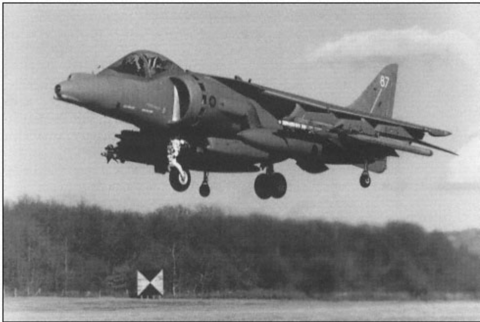
Figure 2.2 British Aerospace Harrier GR7 in hovering flight with its auxiliary air intakes open.
