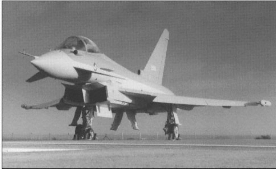
Figure 14.24 The twin intake on the Eurofighter 2000 with the cowl lip deployed in the take-off position on the starboard intake.
